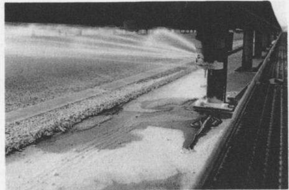
Sprinkler head spraying NaCl over a bridge road surface.
